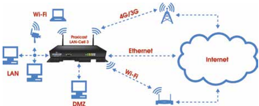
Figure 1: Typical LAN-Cell 3 Network Configuration
